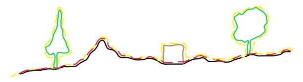
Whereas DTM and DSM data is general represented as a "vector" file, a DEM is generally represented as a "raster" file.
